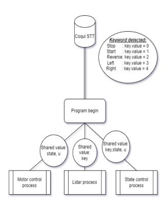
Figure 9 - Flowchart diagram of Python processes to control motors and sensors.
