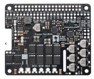
Figure 7 - Dual G2 High-Power Motor Driver from Pololu (24v18 for Raspberry Pi)
